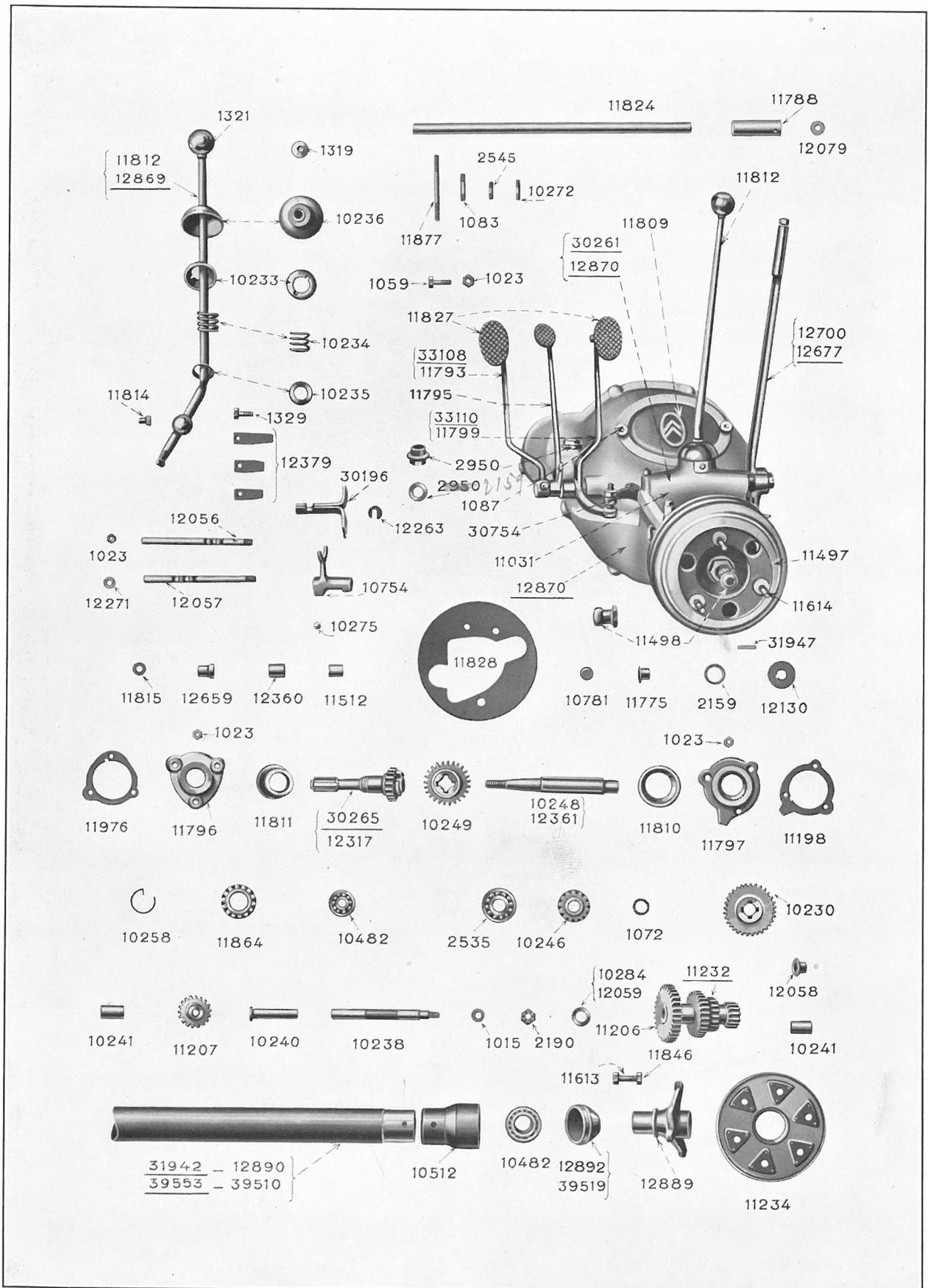
BOITE DE VITESSES (DIRECTION A GAUCHE), TUBE DE RÉACTION
